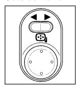
The controls for the outside power mirrors are located on the inside of the vehicle near the driver's side mirror.
